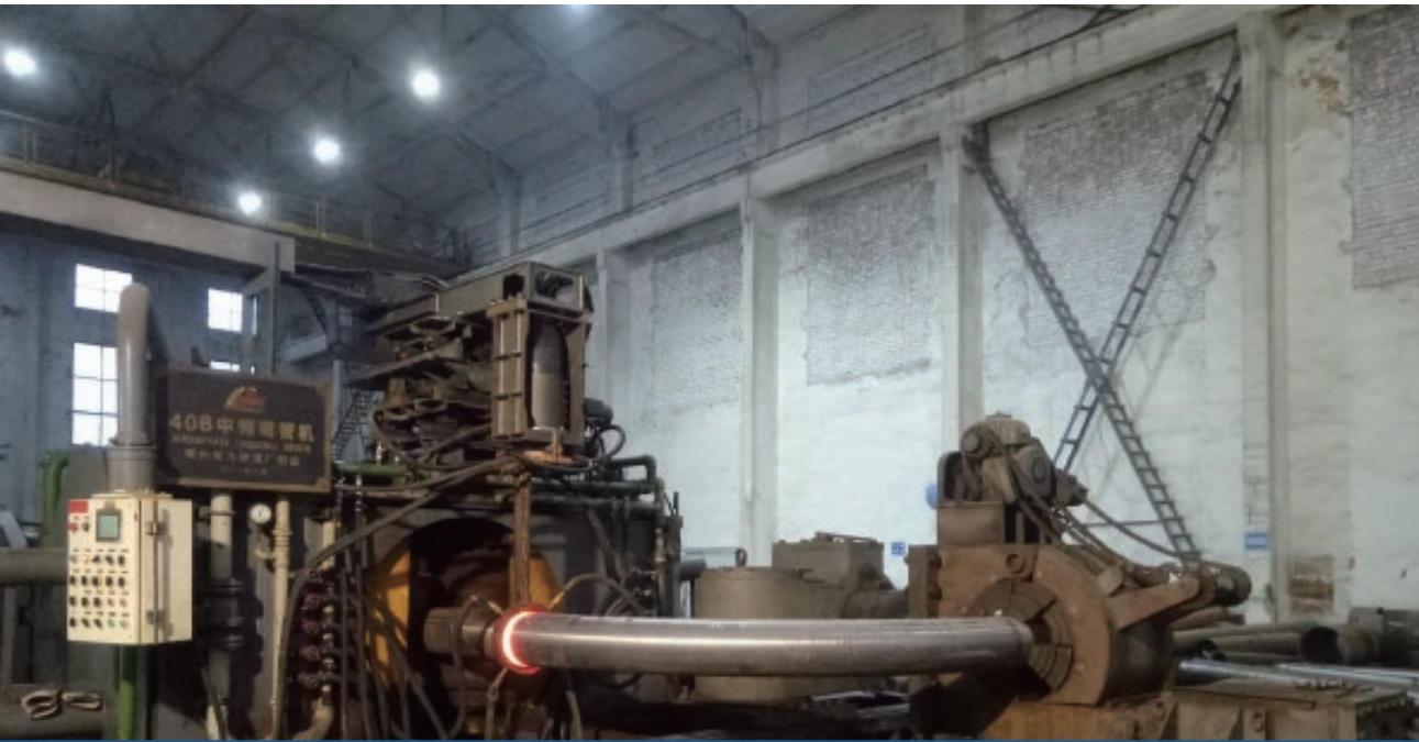
Bending Thick Wall Pipe
