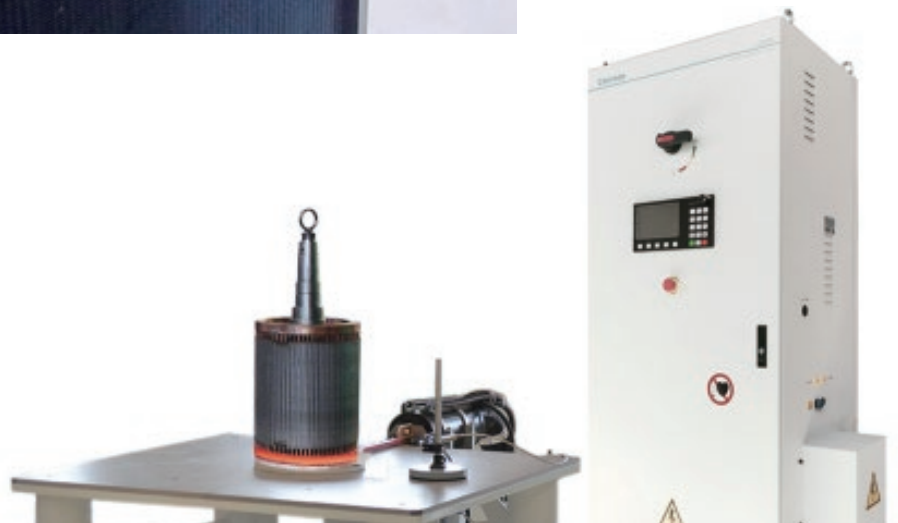
Brazing for Short Circuit Ring
