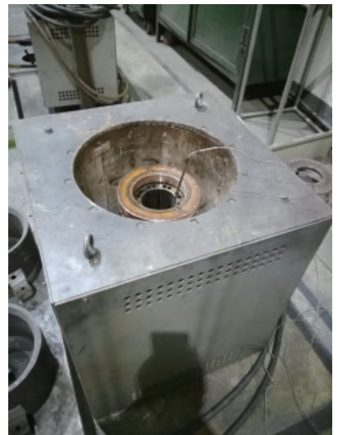
Shrink Fitting for Rotor
