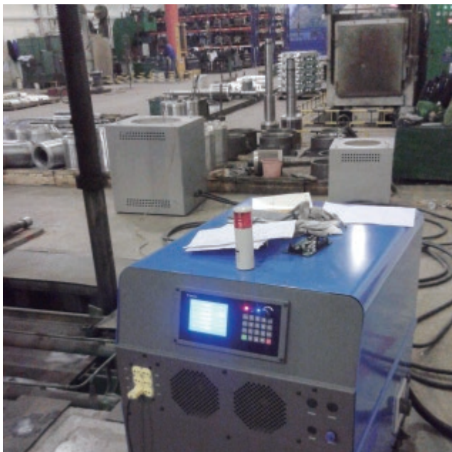
Shrink Fitting for Rotor
