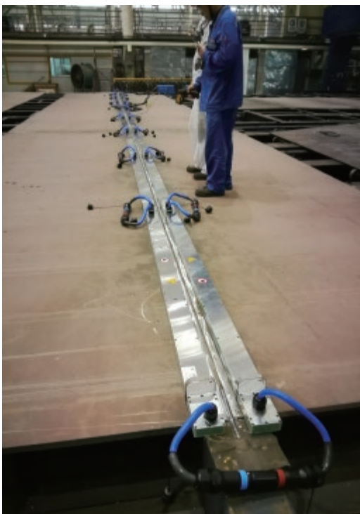
Welding Preheat with flat inductor Shipbuilding
