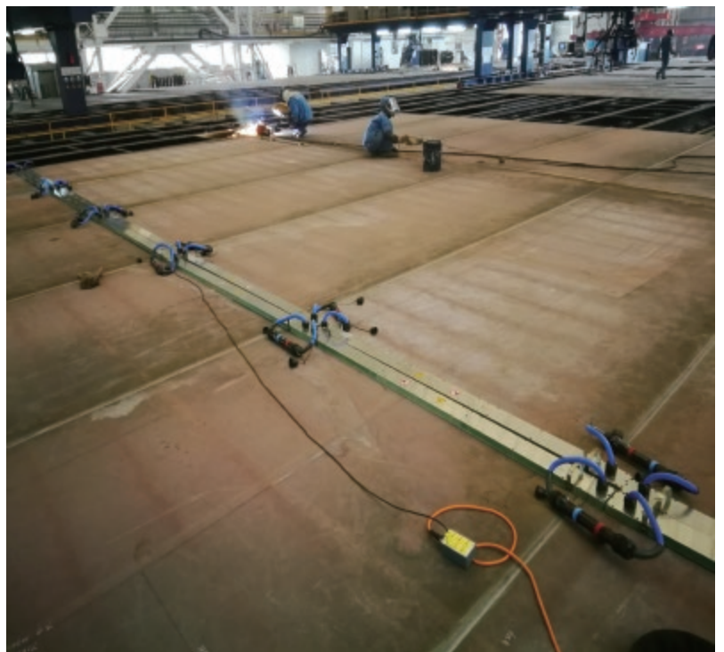
Welding Preheat with flat inductor Shipbuilding
