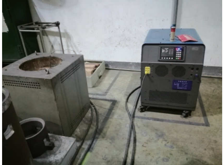
Shrink Fitting for Rotor
