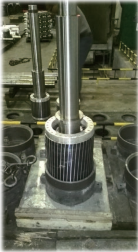
Shrink Fitting for Rotor
