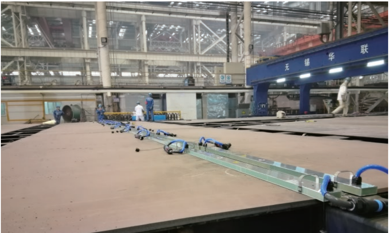
Welding Preheat with flat inductor Shipbuilding
